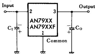
C<sub>1</sub> is set when the input line is long.
