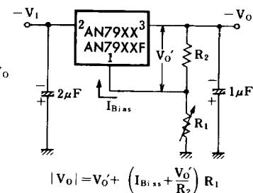
$$|V_o| = V_o' + \left( I_{Bias} + \frac{V_o'}{R_2} \right) R_1$$
