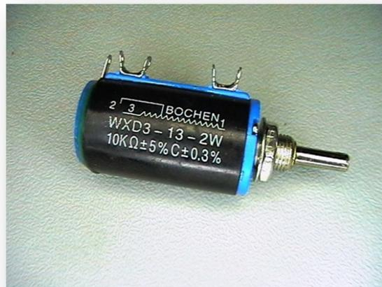
WXD3 -13 potentiometer for oxygen control instrument , nitrogen analyzer, controlled oxygen analyzer to adjust the controller 's maintenance .
